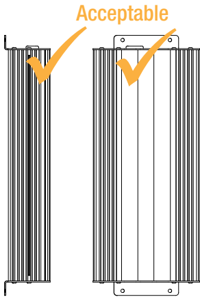
Figure 2.2.1.2 - Vertical mounting is acceptable
