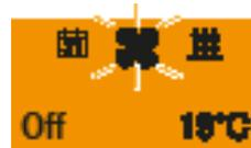
In the Start mask, a flashing fan symbol
